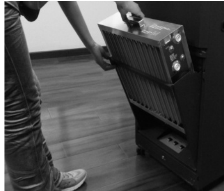
6-4 Removing the cell
