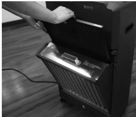
6-5 Replace the activated carbon filter.
